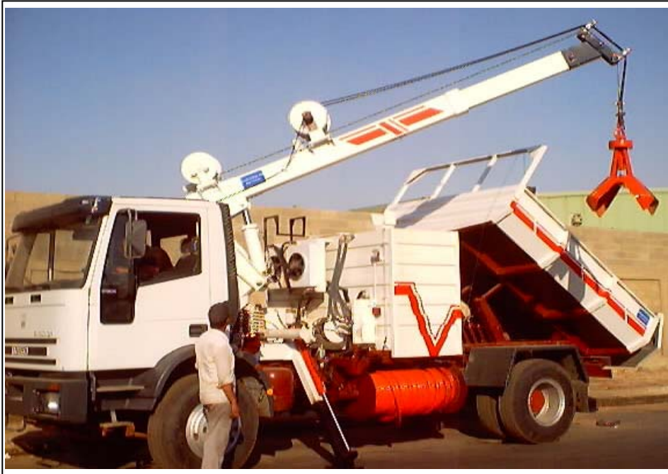
Jetting Catch Basin truck with optional Mechanical cable For sewer cleaning system operated from the Truck powerful engine.
