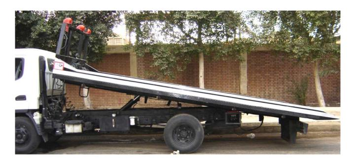
Rescue platform for damaged vehicles that cannot be pulled. The upper platform tilts to 11° then slides down to the ground. The winch on top of the platform pulls the damaged vehicle (5 ton) to the top. The platform returns to its original position, while the damaged vehicle is properly fastened to allow safe long transportation.
