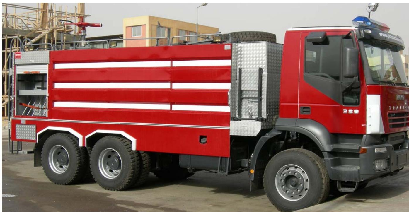
The heavy Fire Fighting Truck can be used to extinguish different types of fires. The truck is equipped with a fire pump, water tank, a water monitor, hose reels and cabinets on the sides. The truck is suitable for working in ports, residential and industrial areas, airports, gas and power stations. The above mentioned can be mounted on Isuzu, Volvo, Mercedes, International, Iveco, Renault and Kamaz chassis. It is designed according to the American NFPA standards.
