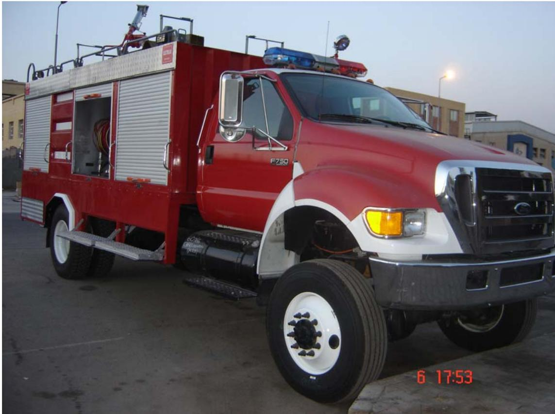
The Multi-Purpose medium Fire Fighting Truck can be used to extinguish different types of fires. The truck is equipped with a fire pump, portable pump, water, foam and dry powder tanks, a water monitor, hose reels and cabinets on the sides. The truck is suitable for working in ports, residential and industrial areas, airports, gas and power stations. The above mentioned is mounted on Ford chassis. It is designed according to the American NFPA standards..
