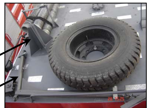
Pic. No.3 showing the carrier when it is stored on the truck roof.
