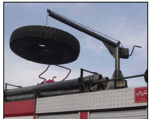
Pic. No.2 showing the carrier during lifting the wheel
