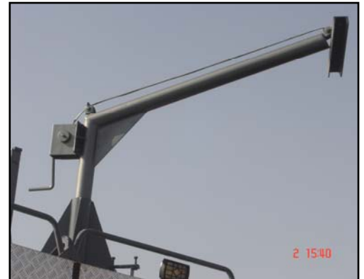
Pic. No.1 showing the carrier ready to lift the wheel
