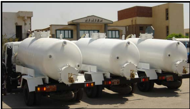
Standard suction truck with optional Mechanical cable for sewer cleaning system operated from the Truck powerful engine.
